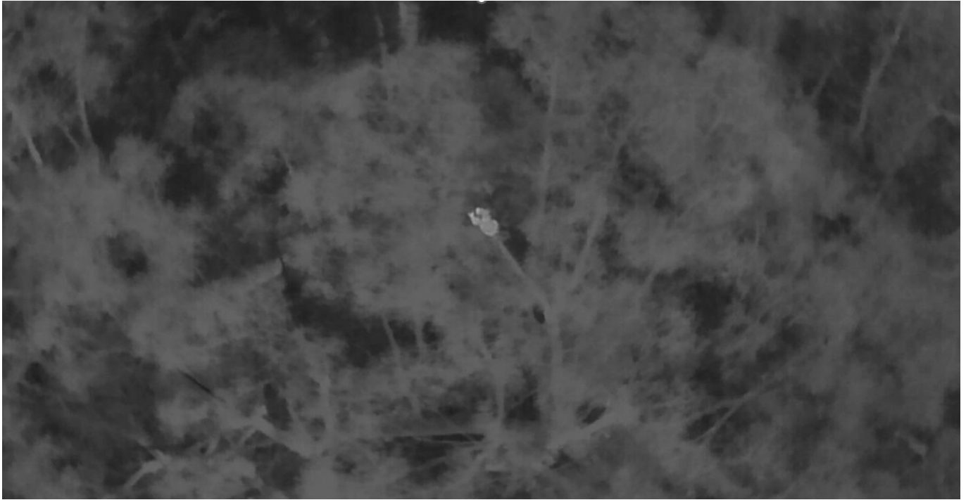
Figure 4. To validate the species identification each drone descend from 65m to an altitude that allowed for an unambiguous view of the target species, in this case, a koala.
